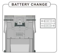
Trun over the car body, and find the battery house. Loosen the screws with a screwdriver. Put 2 AA batteries in the battery house, then tight the screw with a screwdriver.
