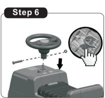
6.Loosen the bolt and nut in the steering wheel first, then place the steering wheel over the J-shaped stick, insert the bolt and tighten the nut with a screwdriver.
