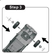
3. Assemble the two front wheels, insert the plastic ring, wheel and washer, tighten using a cotter pin.
