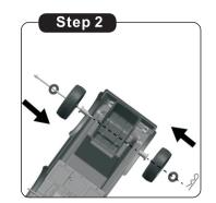
2.Insert the rear wheel axle through washer, wheel, plastic ring into the body, tighten using a cotter pin.
