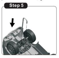
5.Install the J-shaped stick at the assigned location as picture.
